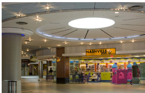
Terminal lighting accounts for 18.4% of electricity use at BNA; to minimize this electricity use, MNAA incorporates natural daylight through large windows and skylights placed throughout the terminal.
