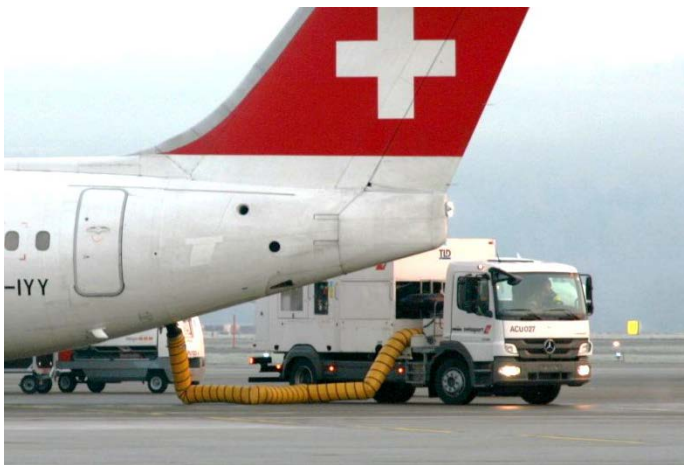
Figure 12 Air Climate Unit (ACU).
